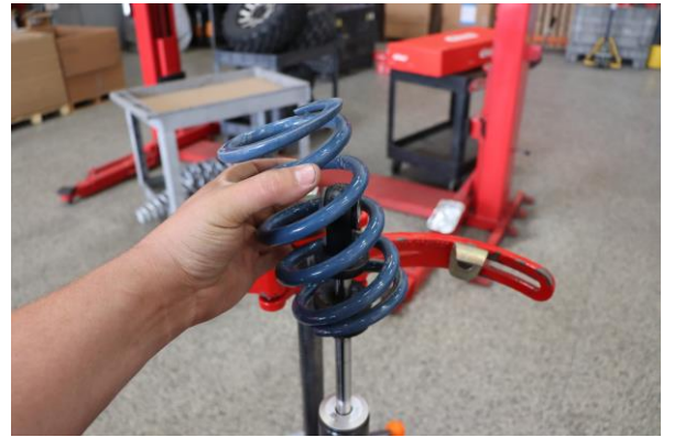
Step 10. Remove the OE tender spring
