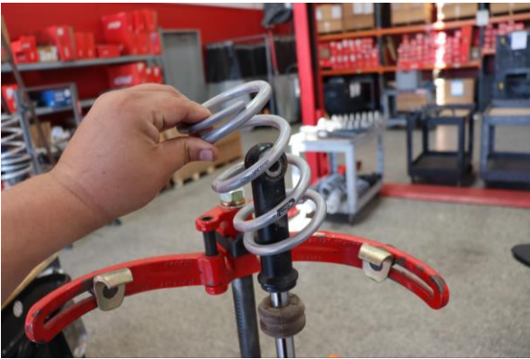
Step 15. Place the shock back in the spring compressor and install the Eibach secondary spring.
