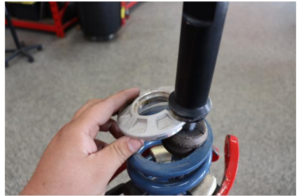
Step 10. Remove the lower spring perch.
