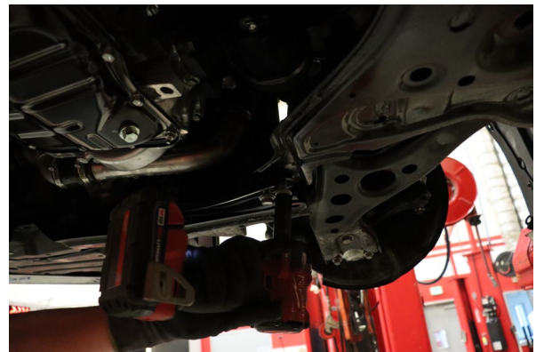
Loosen and remove the bolts for the subframe brace and remove the brace.
