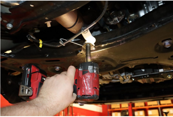
Remove bracket securing the cable to subframe.
