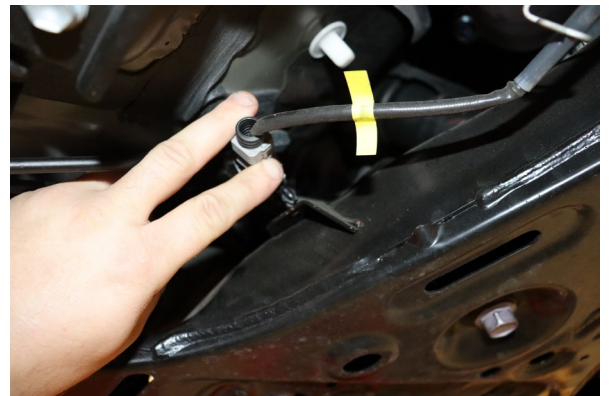
Disconnect cable for o2 sensor from the subframe. You do not need to unplug the cable.
