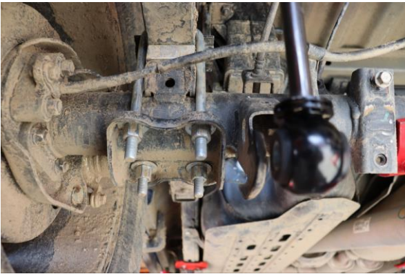
9. Secure the U-bolt bracket with the provided washers and 19mm nuts. Hand tighten each nut first so the U-bolts are showing equal threads on all sides.
