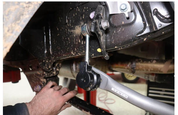
Reinstall the end links to the desired hole on the sway bar.
