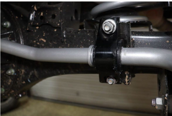
Install the provided sway bar brackets with the OE hardware.
