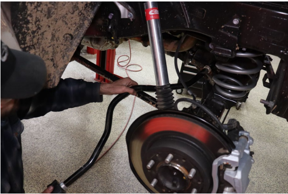
Remove the OE rear sway bar.
