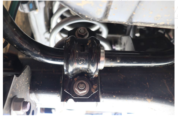
Loosen and remove the OE sway bar brackets.
